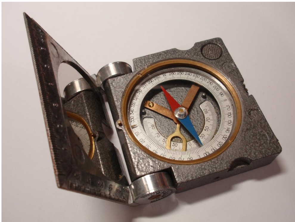
Figure 1. The Clar geological compass which to measure dip and dip direction of geological planes (John V.S 2006)
